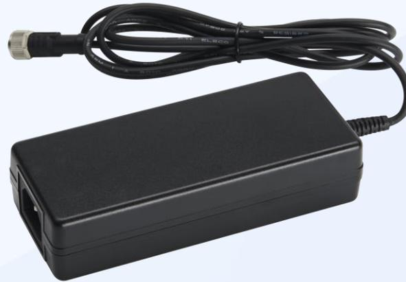
Level VI AC/DC Power Supply Brick, Unsealed. AC Input: 90-264V, 3A; Output: 24V, 3.25A, 78W, -20 TO +55 Degrees C. Requires: Country specific grounded AC line cord
