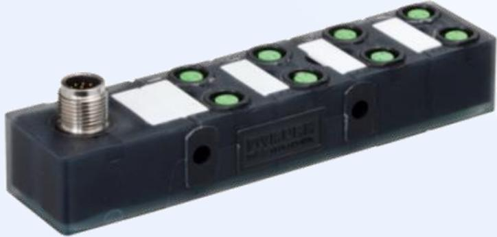
GPIO NPN Breakout Block for use with FXR90. Features 12-Pin M12 GPIO/DC Power Input CONNECTOR, 4x M8 3-Pin GP Inputs, 4x M8 3-Pin GP Outputs.
