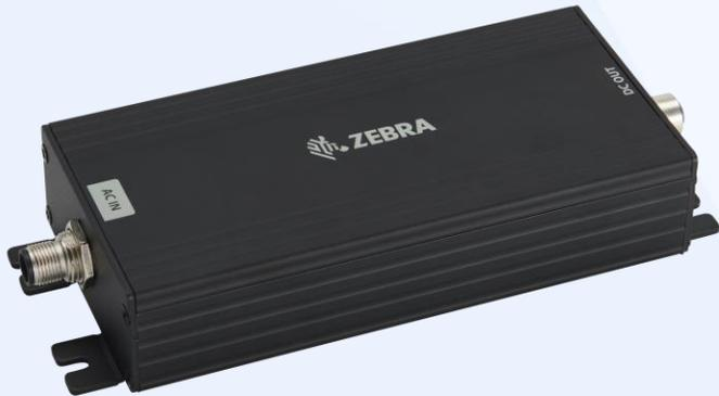
Level VI AC/DC Power Supply Brick, IP67 Sealed. AC Input: 100-240V, 1.4A; DC Output: 24V, 3.75A, 90W, -40 to +65 Degrees C. Requires: Country specific grounded AC line cord
