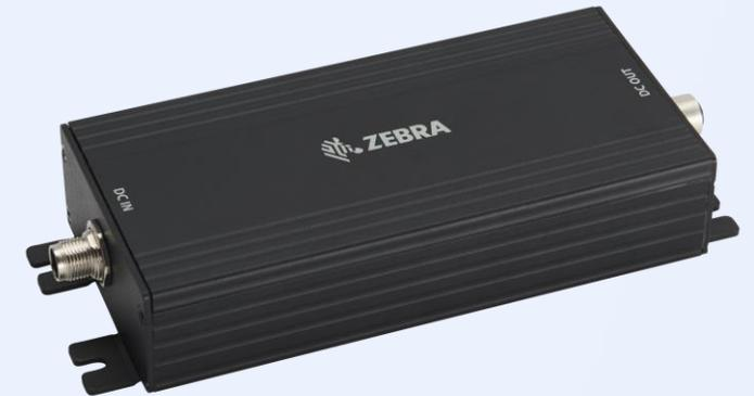
DC/DC Power Supply Brick, IP67 Sealed. DC Input: 9-60V, 17.2A; Output: 24V, 3.75A, 90W, -40 TO +65 Degrees C.
